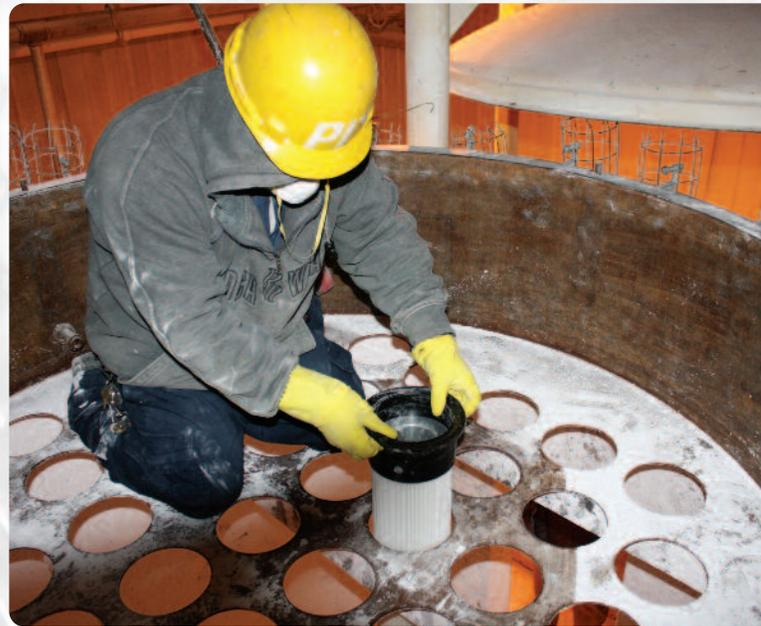
*ProPulse pleated bag filters can be installed in a range of dust-collection applications*
